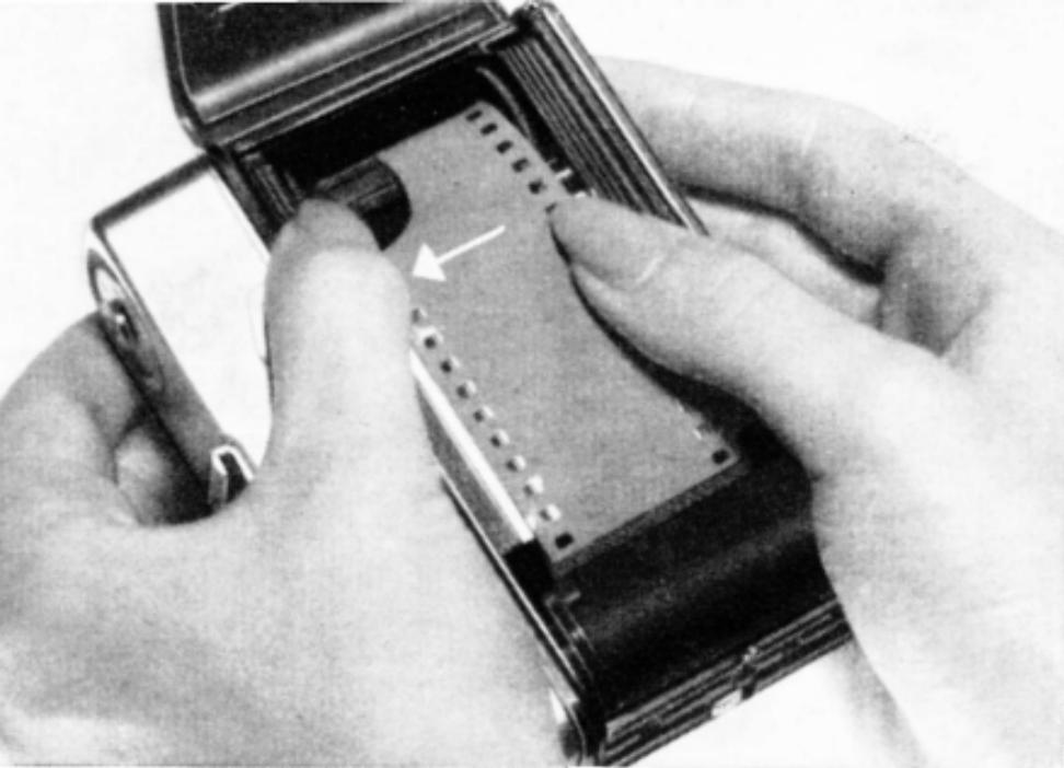
Now wind the film on to the take-up spool until the transport sprocket (15) engages the perforations on both sides. The cut-out knob (17) should be depressed to facilitate this operation. Replace the camera back and lock it.
